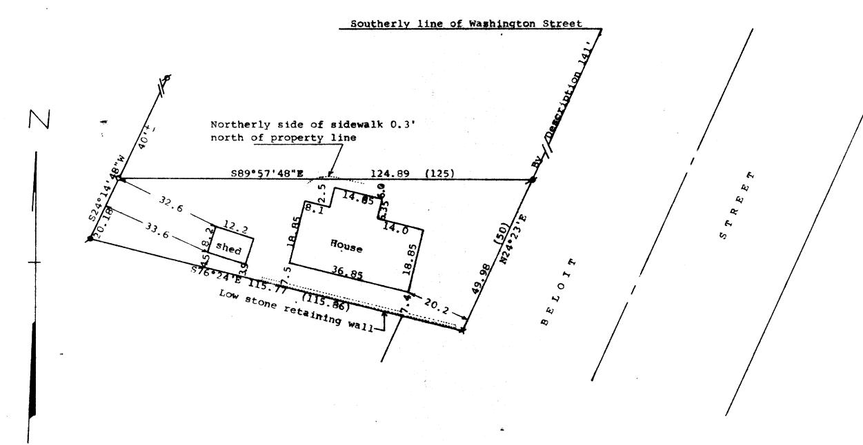
Scale -1" = 20"X= Cross in Concrete Found #= 1" Iron Pipe Found 0 = 3/4" X 24" Iron Pipe Set (00.0) = Recorded distance
